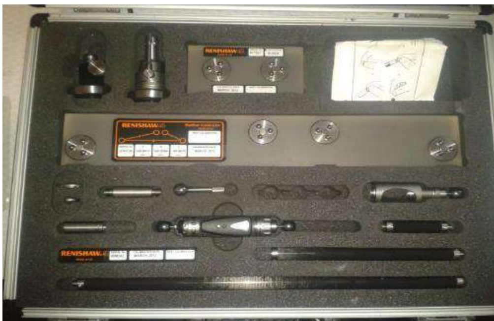
c. Qualitative analysis of the machine tool axis geometry, carried out with the Renishaw QC20 BallBar toolkit.
