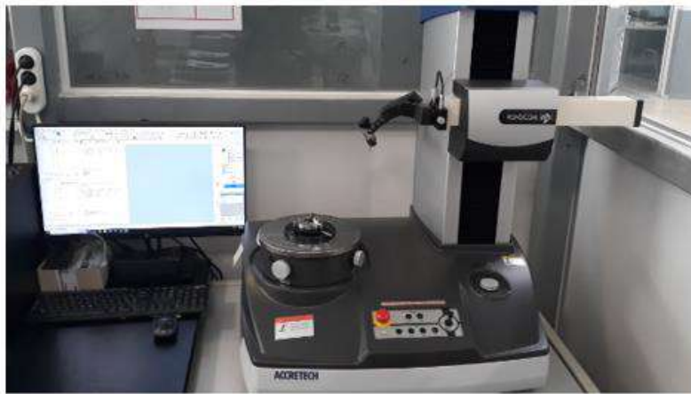
Fig. 3 Accretech form tester (0.5 \mu\text{m} accuracy)
