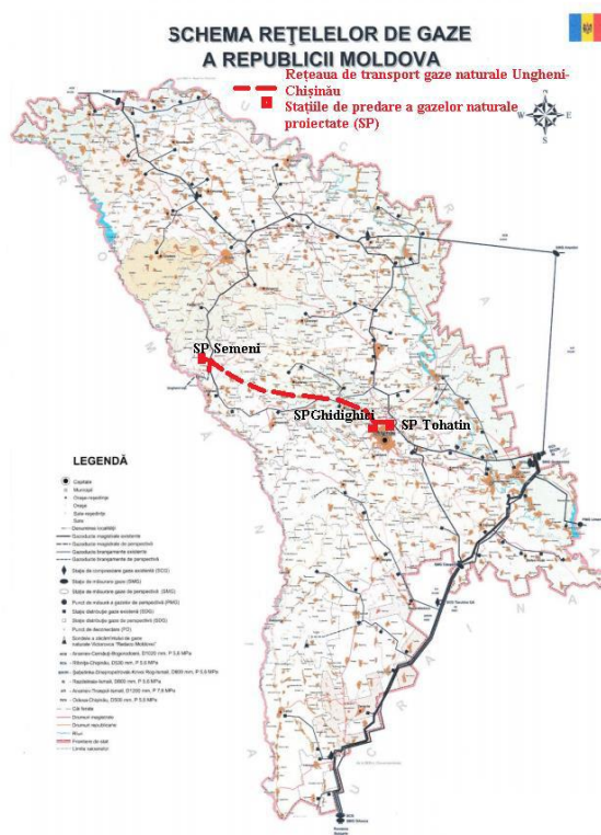
Figure 16. Gas networks in the Republic of Moldova and the extension of the Iași-Ungheni-Chișinău interconnector (Phase II)
