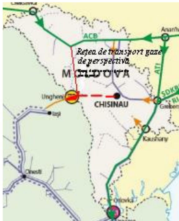
Figure 15. Map of the Republic of Moldova with the main gas transmission interconnection
